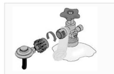
For Quick Connect cylinders, tighten clockwise
