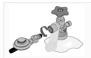
For POL cylinders, tighten anti-clockwise
